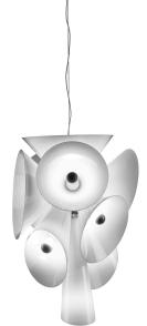
Suspension luminaire providing diffused lighting. Central body in die-cast aluminum and 10 blown glass cones of different sizes. Bayonet-type coupling system of the cones for easy cleaning. Die-cast aluminum ceiling attachment with spherical automatic wire clamp. Polycarbonate rose.
