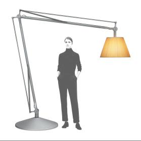
Floor lamp providing direct and diffused light. Acid-etched hand-blown pressed borosilicate glass internal diffuser. Plissé cloth external diffuser. Sand-cast, aluminum diffuser support. Gray painted assembly composed of tubular aluminum arms and tie rods, stainless steel springs, and die-cast aluminum joints. Sand-cast aluminum base with gray painted spun aluminum cover. On the cable there is the electronic dimmer which allows the regulation of light brightness.
